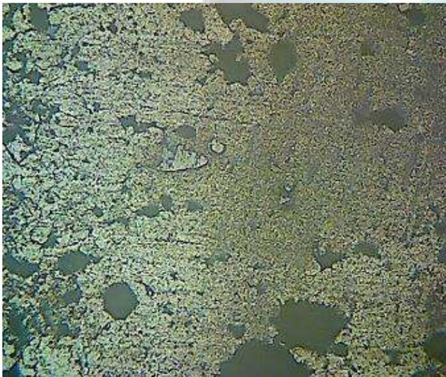
f) AA5083/6% Al<sub>2</sub>O<sub>3</sub>(in μm)/ 4% Al<sub>2</sub>O<sub>3</sub>(in nm)
