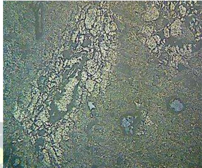
g) AA5083/5% Al<sub>2</sub>O<sub>3</sub>(in μm)/ 5% Al<sub>2</sub>O<sub>3</sub> (in nm).
