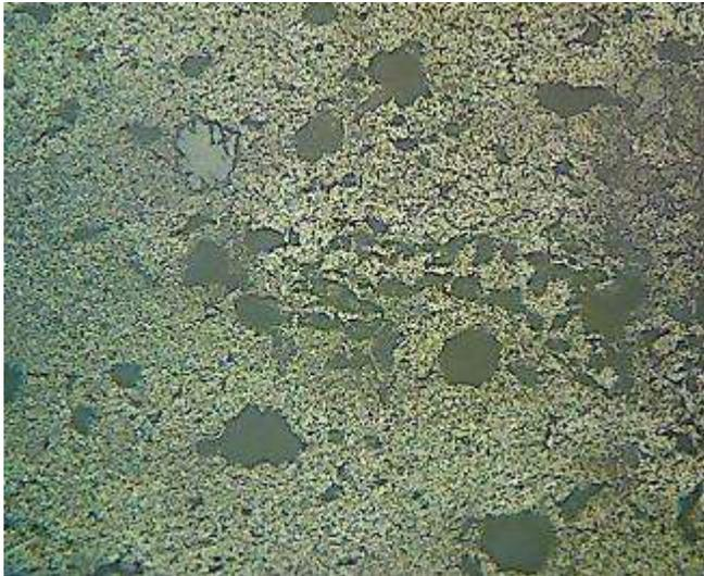
e) AA5083/7% Al<sub>2</sub>O<sub>3</sub>(in μm)/ 3% Al<sub>2</sub>O<sub>3</sub>(in nm)
