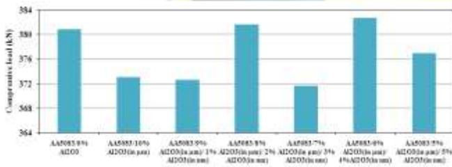
FIGURE 1: Compressive strength of various compositions
