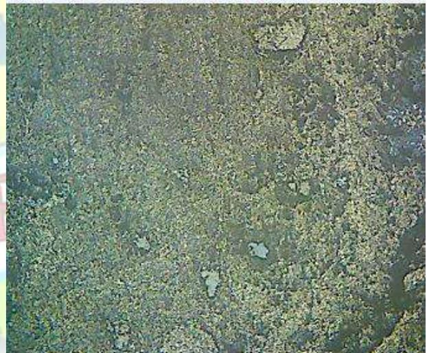
d) AA5083/8% Al<sub>2</sub>O<sub>3</sub>(in  $\mu\text{m}$ )/ 2% Al<sub>2</sub>O<sub>3</sub>(in nm)
