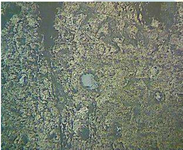
b) AA5083/10% Al<sub>2</sub>O<sub>3</sub>(in  $\mu\text{m}$ )
