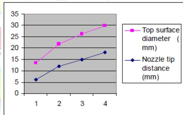
Graph Shows The Relationship Between Nozzle Tip Distance And Top Surface Diameter Of Hole At A Set Pressure 6.5 Kg/ cm<sup>2</sup>
