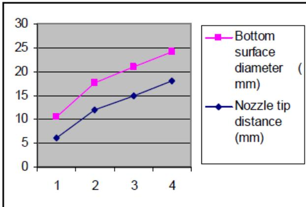
**Graph Shows The Relationship Between Nozzle Tip Distance And Bottom Surface Diameter Of Hole At A Set Pressure 6.5 Kg/ cm<sup>2</sup>**
