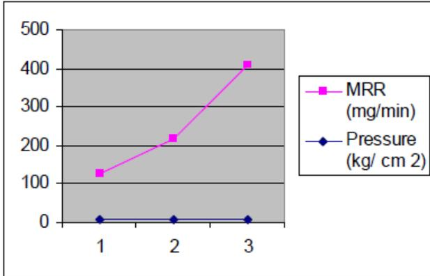
Graph Shows The Relationship Between Pressure And Material Removal Rate (MRR) At Thickness 8 mm And NTD 12 mm
