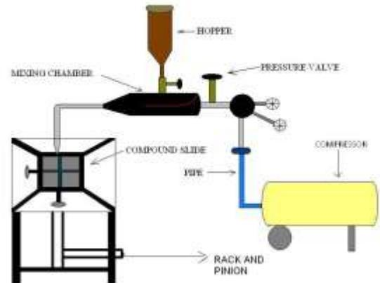
The compressed air from the compressor enters the mixing chamber partly pre-filled with fine grain abrasive particles. The vortex motion of the air created in the mixing chamber carries the abrasive particles to the nozzle through which it is directed on to the work-piece. The nozzle and the work-piece are enclosed in a working chamber with a Perspex sheet on one side for viewing the operation
