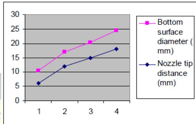
Graph Shows The Relationship Between Nozzle Tip Distance And Bottom Surface Diameter Of Hole At A Set Pressure Of 5.5 Kg/ cm<sup>2</sup>
