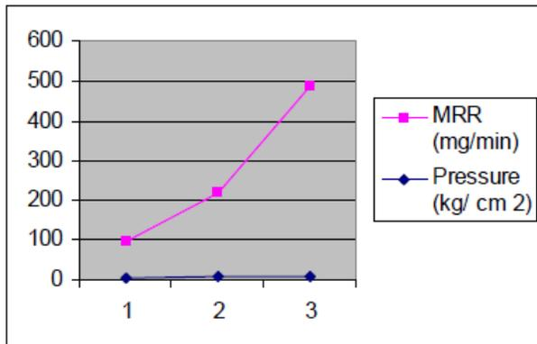
Graph Shows The Relationship Between Pressure And Material Removal Rate (MRR) At Thickness 12 mm And NTD 12 mm
