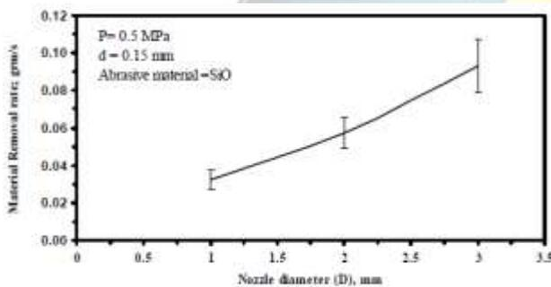
**Effect Of Nozzle Diameter (D) On The Material Removal Rate Of The Glass**
