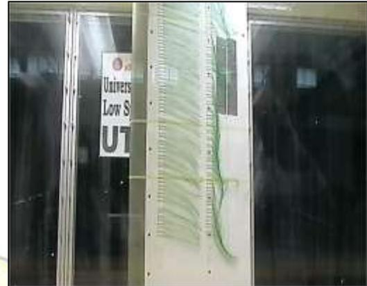
b) Tuft Test at  $V = 10$  m/s Angle of
