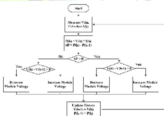
Fig.4. Flowchart of P&O Algorithm
