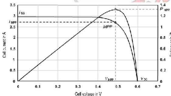
Fig.3. I-V Characteristics of PV cell
