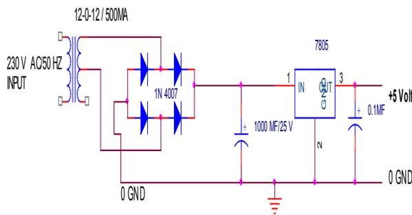
Fig No. 1 Circuit Diagram of Power Supply
