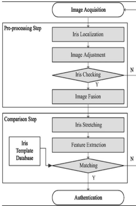
Fig. 1. Flow Diagram of proposed scheme
