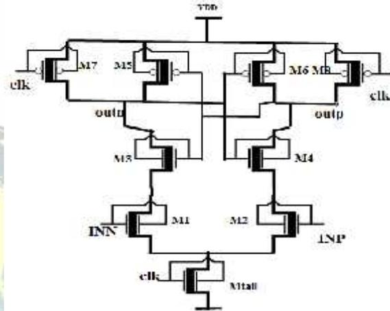
Fig. 1 FinFET based Single tail comparator
