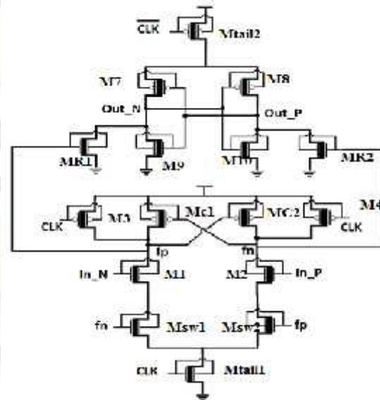
Fig. 3 FINFET based Proposed dynamic double tail high speed comparator
