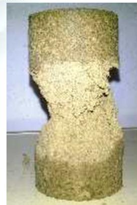
Fig - 2 Failure pattern observed for soil sample 1 treated with molasses
