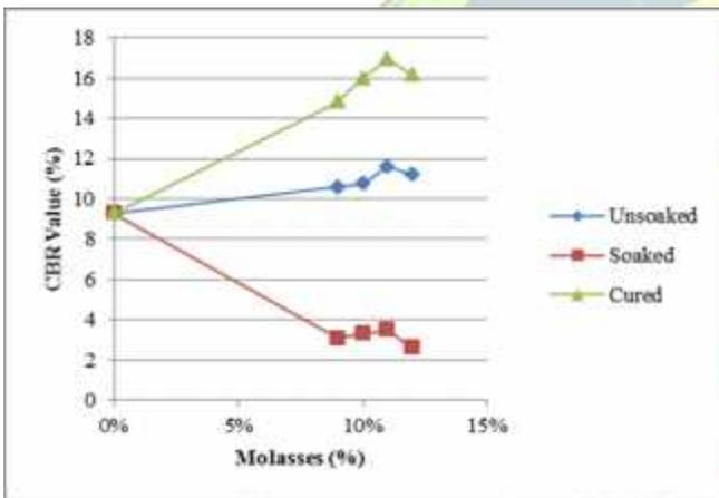
Fig - 6 Comparison of variation of influence of molasses treatment on CBR values for soil sample 2
