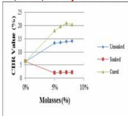
Fig - 5 Comparison of variation of influence of molasses treatment on CBR values for soil sample 1
