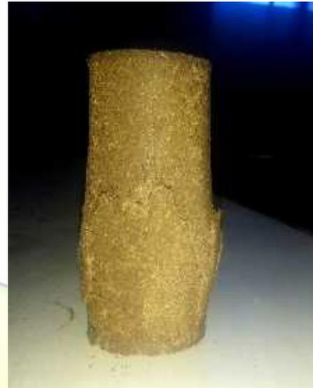
Fig - 4 Failure pattern observed for soil sample 2 treated with molasses
