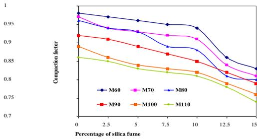
Fig. 3. Workability through compaction factor values
