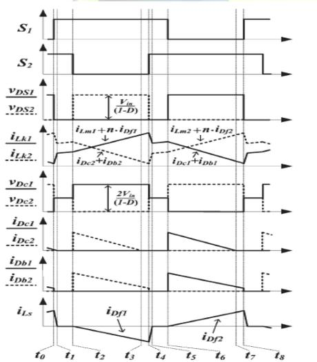
Fig.4. Steady waveform of the proposed converter in CCM
