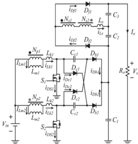
Fig.3. Equivalent circuit of the proposed converter
