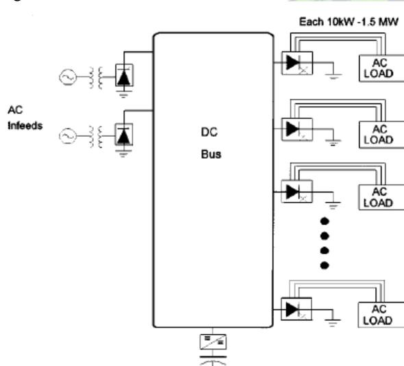
Fig 9. DC system with capacitive energy storage added to the dc system through a dc-to-dc converter.
