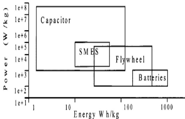
Fig 1. Specific power versus specific energy ranges for near-to-midterm technology.
