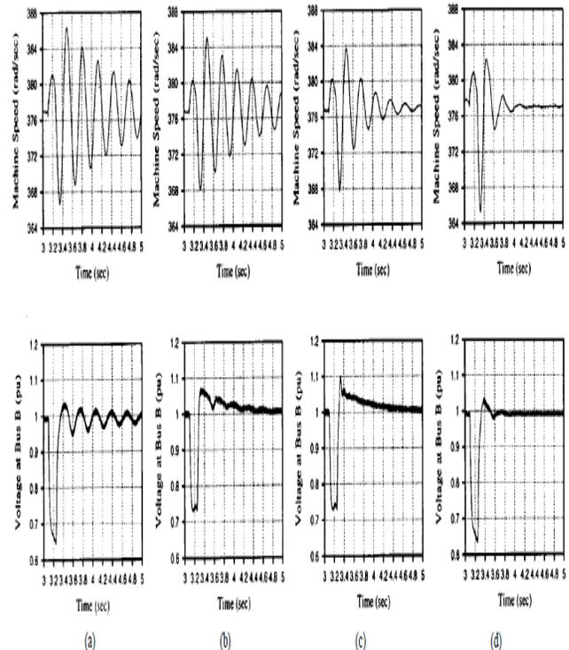
Fig 8. StatCom/SMES dynamic response to ac system oscillations. (a) No compensation. (b) StatCom only at tieline bus. (c) StatCom/SMES tieline bus. (d) StatCom/SMES at generator
