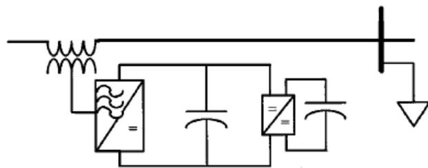
Fig 10. Dynamic voltage restorer (DVR) with capacitor storage
