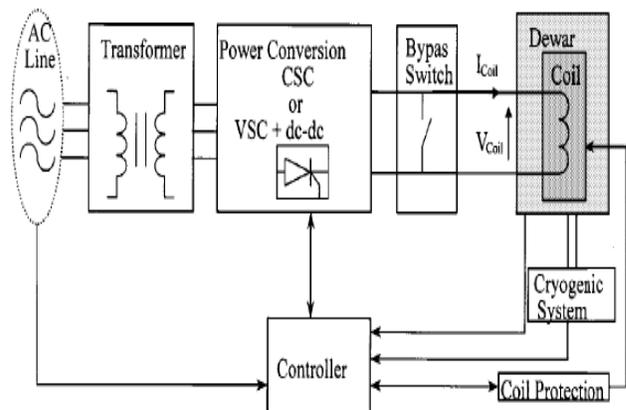
Fig 2. Components of a typical SMES system
