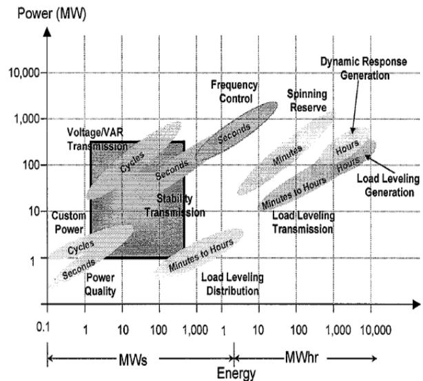
Fig 4. Energy-power characteristics of potential SMES applications
