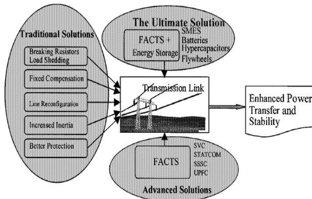
Fig 7. The ultimate solution: FACTS+ESS.
