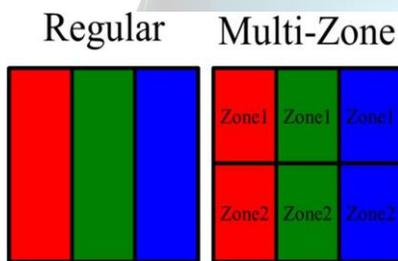
Fig. 2. Comparison of pixel layout of a regular panel and a 2D1G panel.
