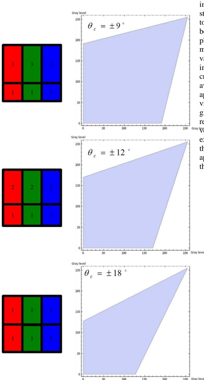
Fig. 6. Limitation of MZ-DCR method corresponding to the gray level of each pixel and the ratio between main region and sub region
