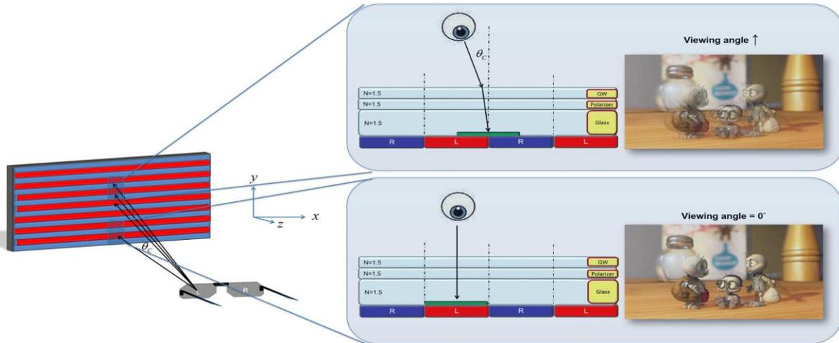
Fig. 1. User watches a patterned retarder display in vertical direction. The images at the right side show main components of the pattern retarder display and the corresponding images at different viewing angle.
