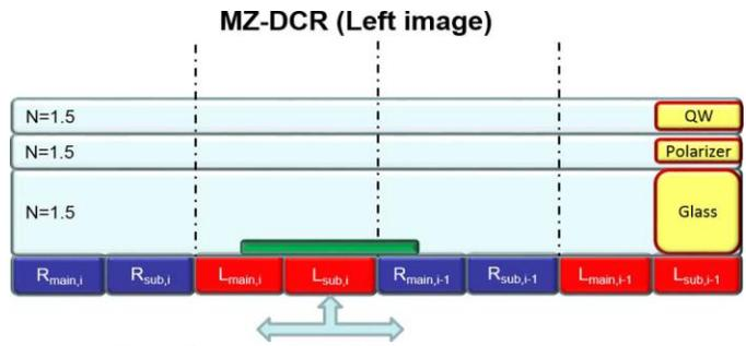
Fig. 4. Principle of MZ-DCR method in left image.
