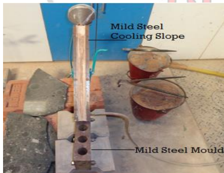
Fig. 9: Mild Steel Cooling Slope
