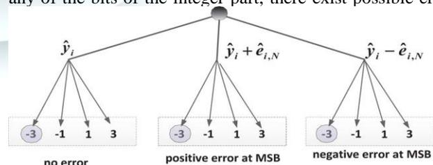
Fig. 1 Tree structure with erroneous children nodes using 16-QAM.
