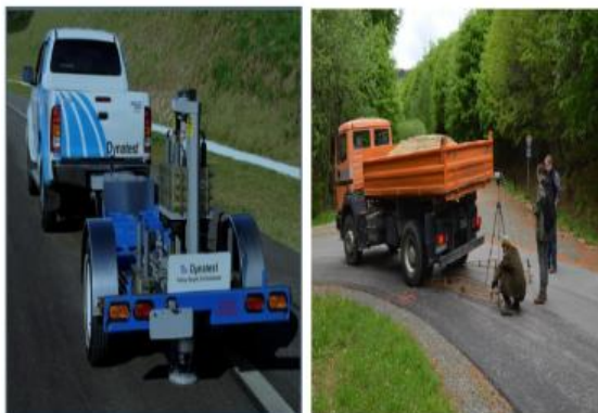
Figure 1. Falling Weight Deflectometer (left) and Improved Benkelman Beam Apparatus (right) in action.
