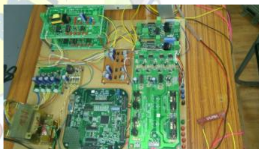
Fig.7.Experimental setup for the single – phase thirteen - level PWM inverter.
