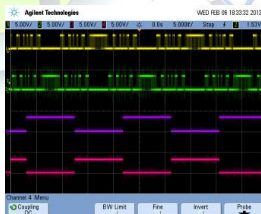
Fig.8.PWM signals for S1, S2, S3 and S4.
