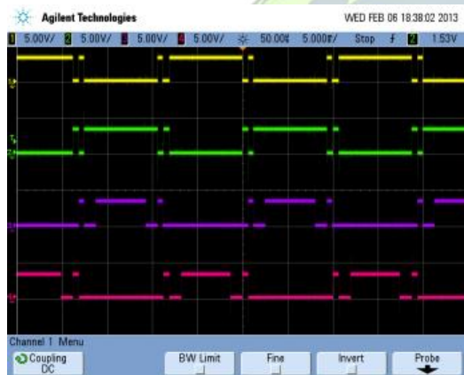
Fig.10.PWM signals for S6, S7, S8 and S9.
