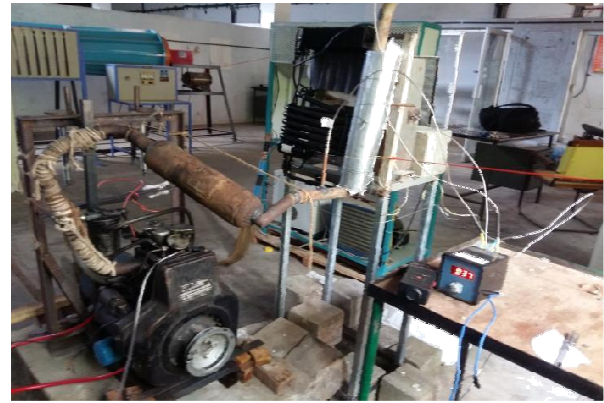
Fig 5. Absorption refrigerator adapted to engine exhaust system.
