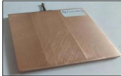
Fig 3: Photograph of the vapor chamber heat spreader
