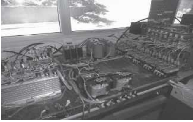
Fig. 15. Laboratory prototype of UPF converter used to compare the ACC and HCC methods.
