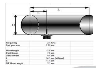
**3. Drilling holes for the N connector and bolts:** Using a drill (or a nail in combination with a hammer if an electric drill isnot available), drill a hole large enough to insert the N-connector and four holes for the securing bolts.
