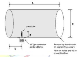
**1. Prepare the can:** Obtain a clean, empty can (with one end open) of radius of 3.65cm - 4.67cm. It might be necessary toremove the lip at the edge of the can so that it does not interfere with reception. Here: r = 3.65cm
