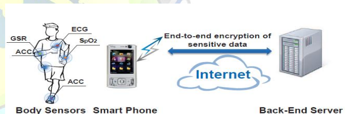
Fig 1 An Example 3-Tier WBAN System
