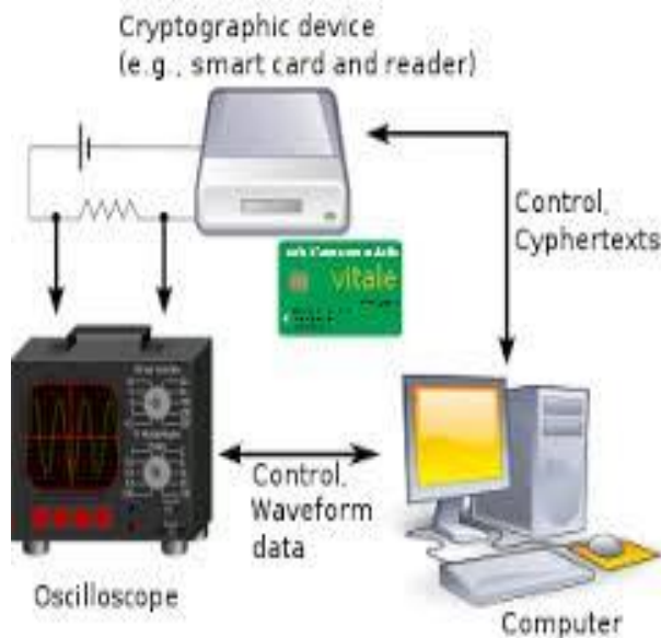
Fig. 6. Power Analysis Attack
