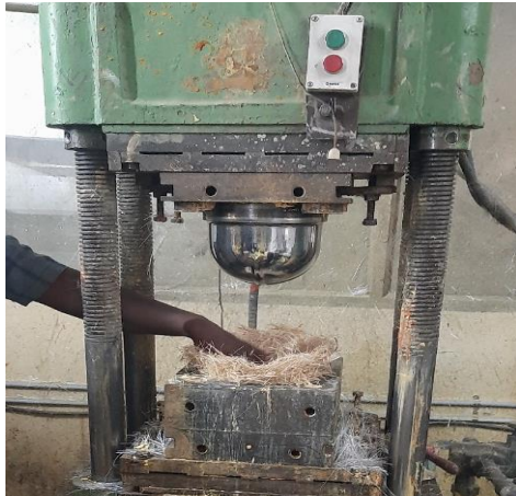
Figure 18 Compression moulding machine
