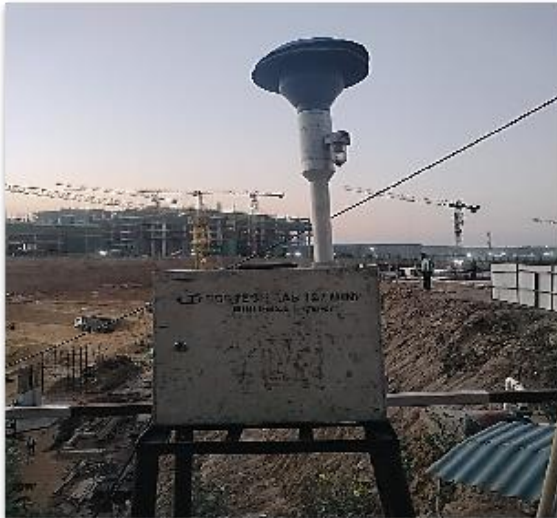
Figure 1: Depicts the PM10 sampler, which is employed to monitor air quality by capturing PM10 particles from the atmosphere.
