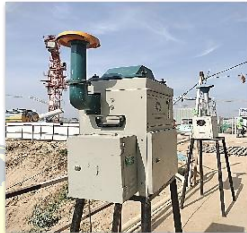
Figure 2: Represents the PM2.5 sampler, highlighting its role in assessing air quality and understanding pollution impacts.
