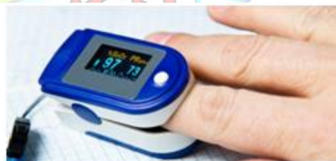
Figure 7c SPO2 and Heartbeat Sensor Positioning and sensor model
