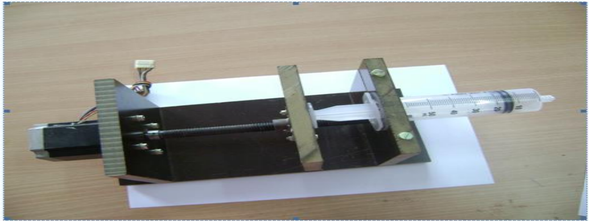
Figure no 7 c Mechanical model with syringe Interface
