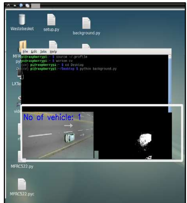
Figure 5: Background Subtraction and counting the number of vehicles
