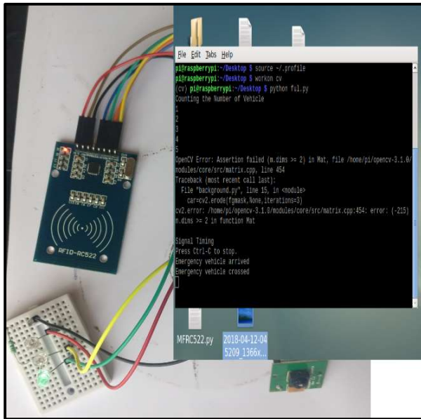
Figure 7: Depending upon the vehicle count Signal timing is adjusted
