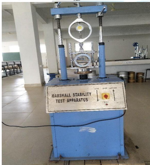
Fig 4.1 Marshall Apparatus
