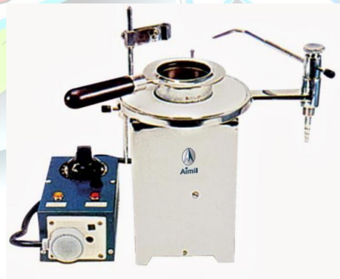
Fig 3.6 Flash and Fire Point Test Apparatus
