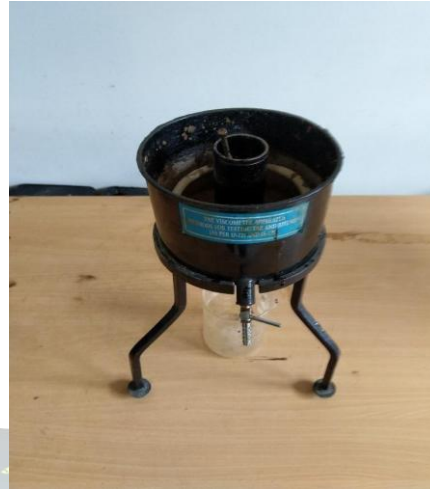
Fig 3.5 Viscosity Test Setup
