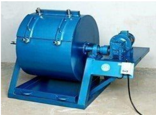
Fig 3.1 Los Angeles Abrasion Test Setup
