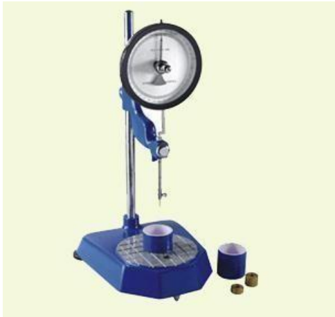
Fig 3.4 Penetration Test Setup
