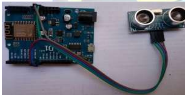
Fig 17. ESP8266 with HCSR04
