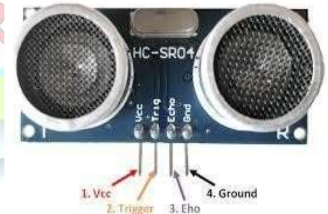
Fig 3. HC-SR04 Ultrasonic Sensor
