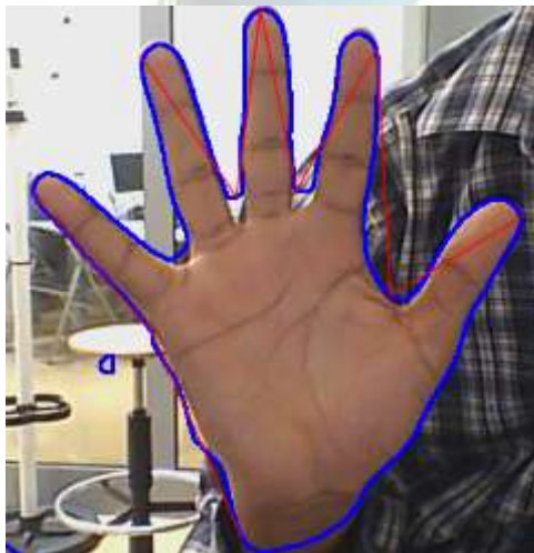
Figure 4: An approximate polygon to extract the convex hull (red line)
