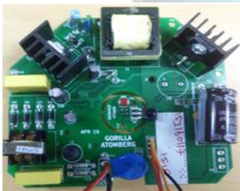
Fig 1. Electronics in a BLDC Fan motor
