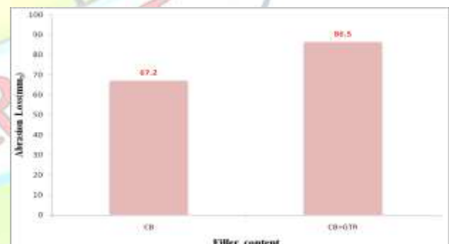
Figure 6. Abrasion loss of NBR composites.
