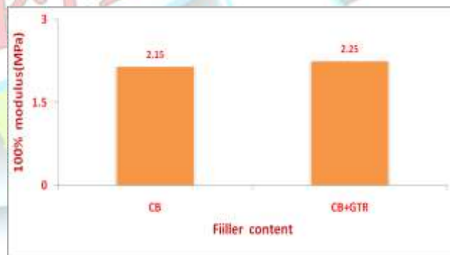
Figure 3. 100% modulus of NBR composites.
