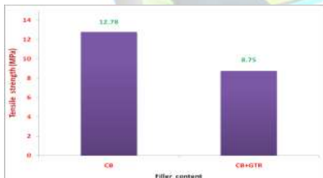
Figure.1. Tensile strength of NBR composites.
