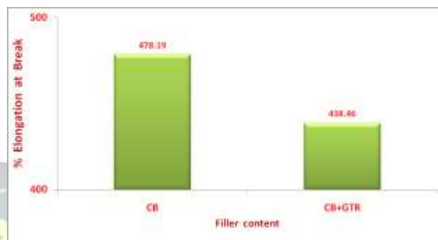
Figure.2. Elongation at break of NBR composites.
