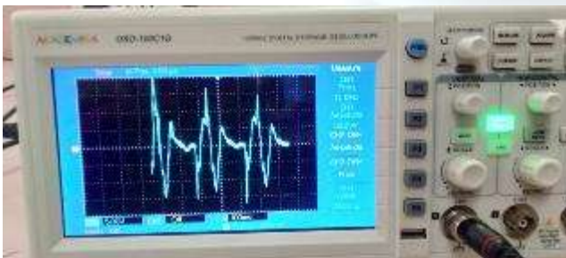
Fig 8: Piezoelectric output on DSO when non-uniform vibration is applied
