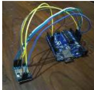
Fig 7: Interfacing of LoRa with Arduino
