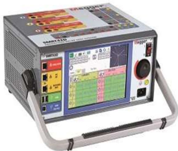
Fig. 2. Relay test kit (Model:SMRT43D of Megger Company)
