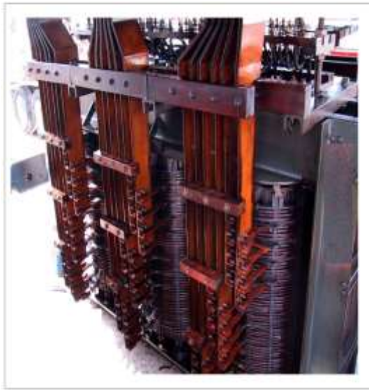
Fig. 3 Internal parts of a Transformer
