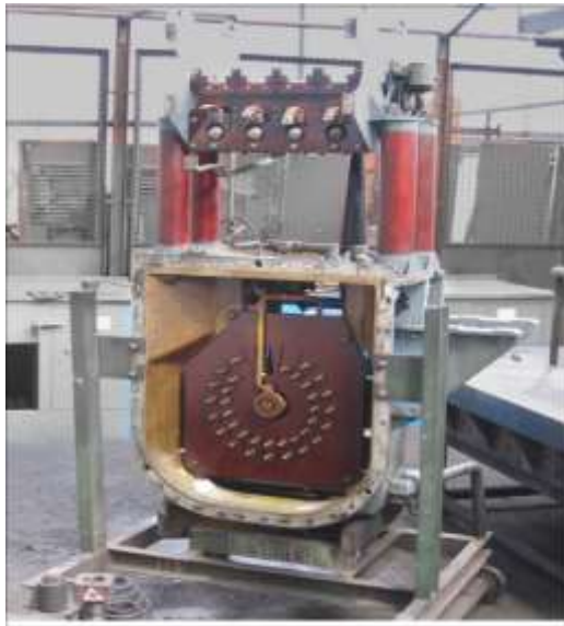
Fig. 4 Off-Circuit Tap switch
