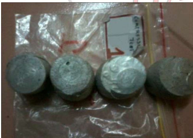
Compression test specimen
