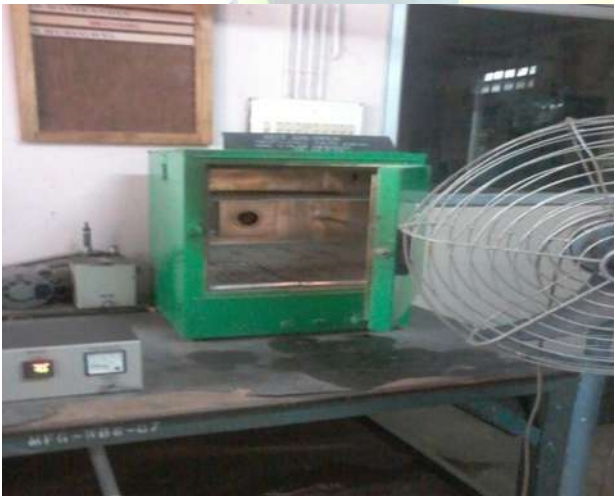
Muffle furnace used for preheating
