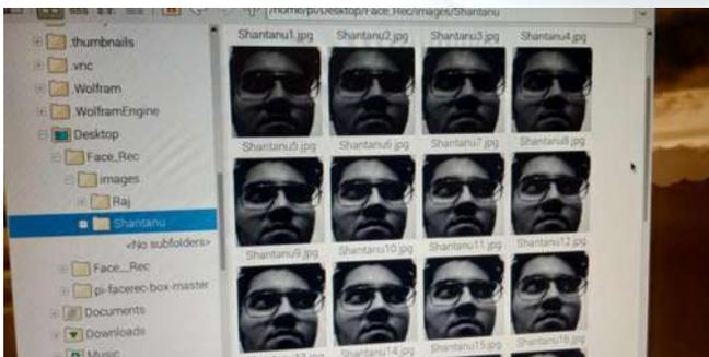
Training the dataset also took very less time when compared to the other models we used. It took few minutes to train the model. We trained the model in **Raspberry Pi**, if we train the Inception model on Raspberry Pi then it takes about an hour to train. Therefore, The LBPH algorithm was much more efficient in training. This is why it is still widely used due to its computational simplicity and discriminative power in many different applications.
