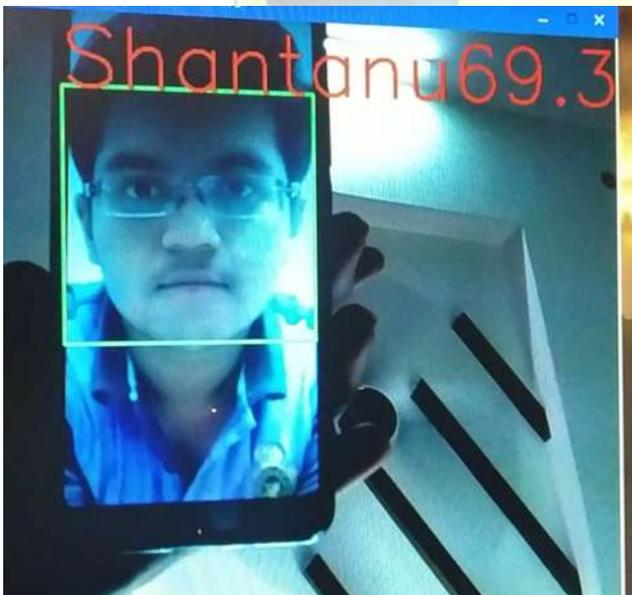
This could be a major security concern for the projects that have been made based on LBPH algorithms. So, we added something which cannot be easily tricked by someone i.e., Fingerprint. A fingerprint scanner will act as
