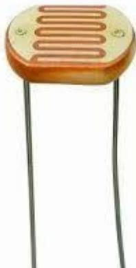
LDR sensor has two cadmium sulphide photoconductive cells (cdS) with spectral response similar to that of the human eye. The cell resistance will fall with the increasing light intensity. Its application includes smoke detection, automatic
