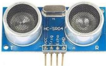
*Ultrasonic sensors module includes ultrasonic transmitters, receiver and control circuit. It provides*
