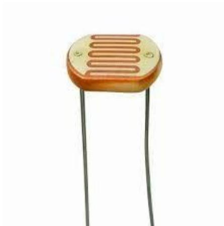
LDR sensor has two cadmium sulphide photoconductive cells (cdS) with spectral response similar to that of the human eye. The cell resistance will fall with the increasing light intensity. Its application includes smoke detection, automatic
