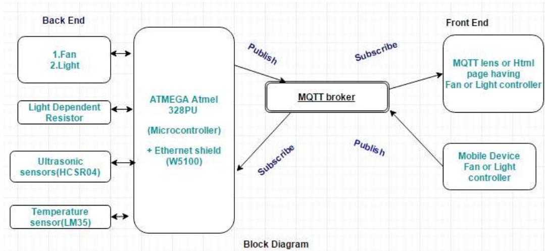
In the above block diagram, there are three parts which as follows:
