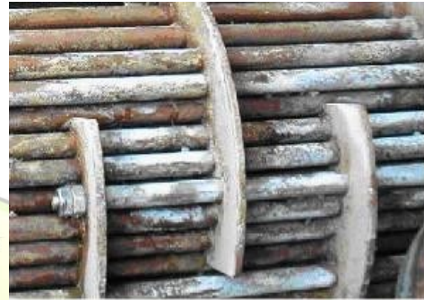
Figure 2. Scaling or Crystallization Fouling
