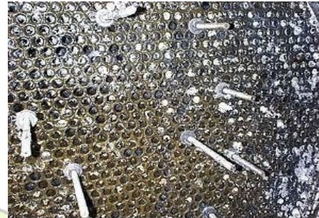
Figure 6. Freezing Fouling
