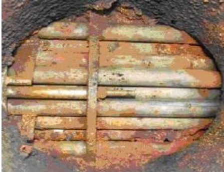
Figure 4. Corrosion Fouling
