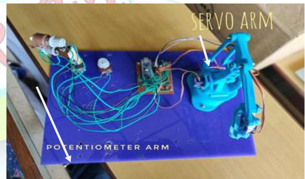
Fig. 5. Servo arm and Arduino Nano board with potentiometer
