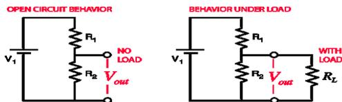
$$V_{out} = V_1 \frac{IR_2}{I(R_1 + R_2)} = \frac{V_1 R_2}{(R_1 + R_2)}$$
