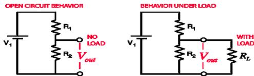
$$V_{out} = V_1 \frac{R_2}{R_1 + R_2} = \frac{V_1 R_2}{R_1 + R_2}$$
