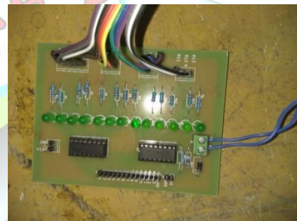
Figure 3. Relay interfacing circuit board
