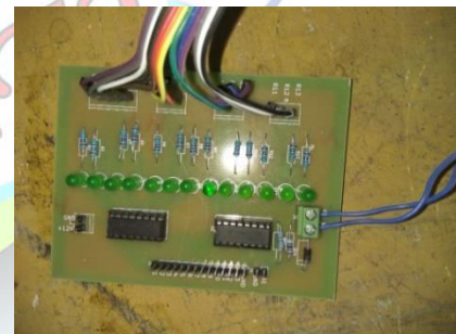
Figure 3. Relay interfacing circuit board
