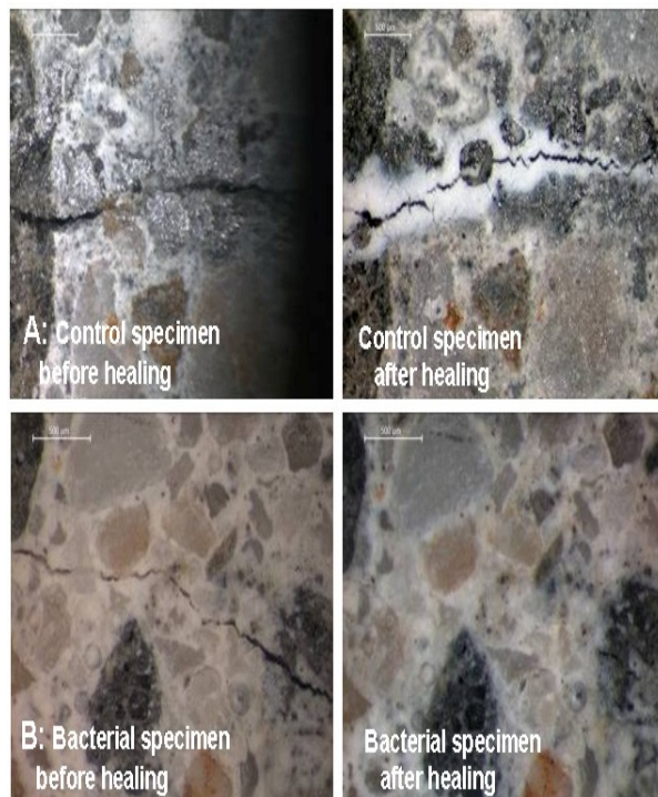
Figure 4. Light microscopic images (40 times magnification) of pre-cracked control (A) and bacterial (B) concrete specimen before (left) and after (right) healing (2 weeks submersion in water). Mineral precipitation occurred predominantly near the crack rim in control but inside the crack in bacterial specimens. Efficient crack healing occurred in all six bacterial and two out of six control specimens.
