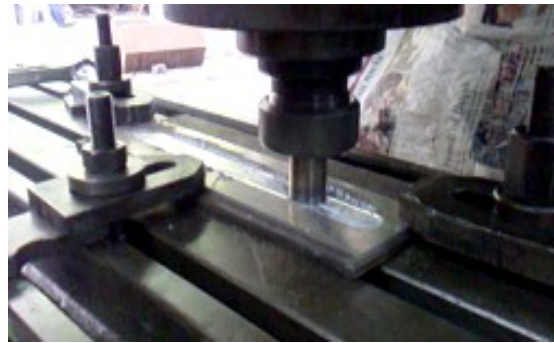
Fig.2 Experimental setup of FSP
