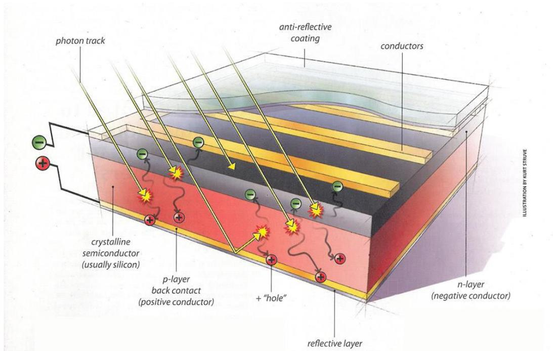
The electricity output of the solar cells per unit radiation is called solar cell efficiency. Present day solar cells are made up of different materials and the efficiencies are ranging between 10-23% for terrestrial applications. The solar cells used for space applications are highly expensive and are made of multi junction technology with the efficiencies between 36-42%.
