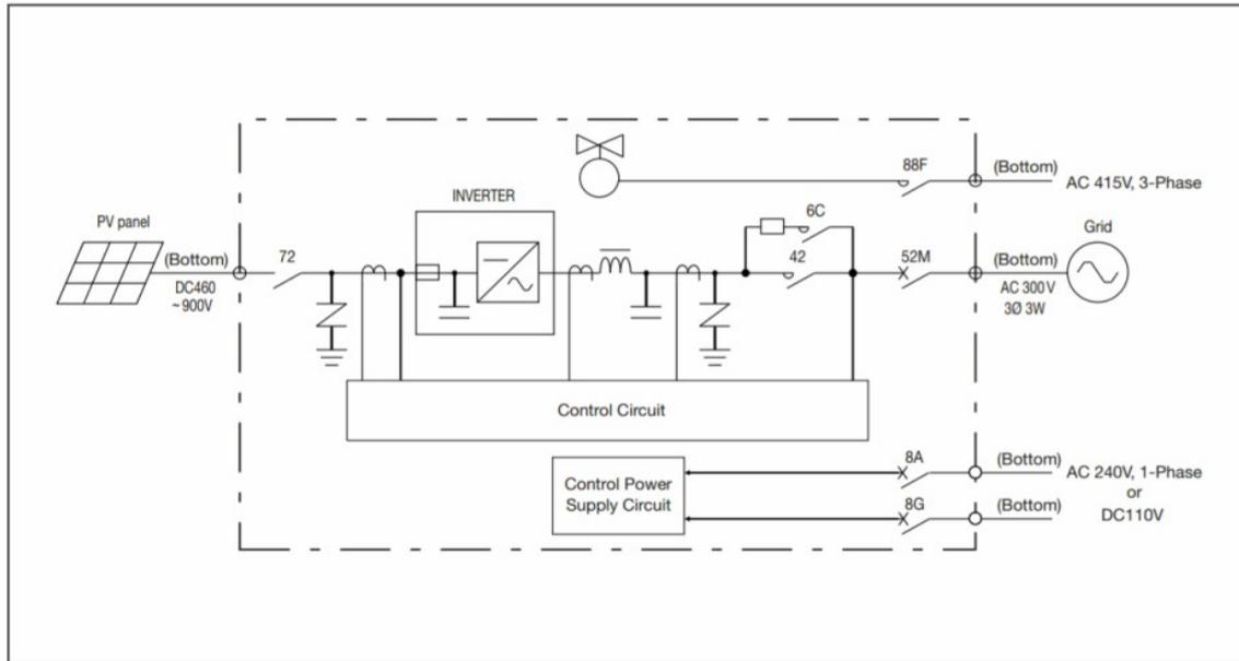
The DC voltage from the PV array, which is of 750V, is converted to 350V AC by the inverters present in the inverter rooms.
