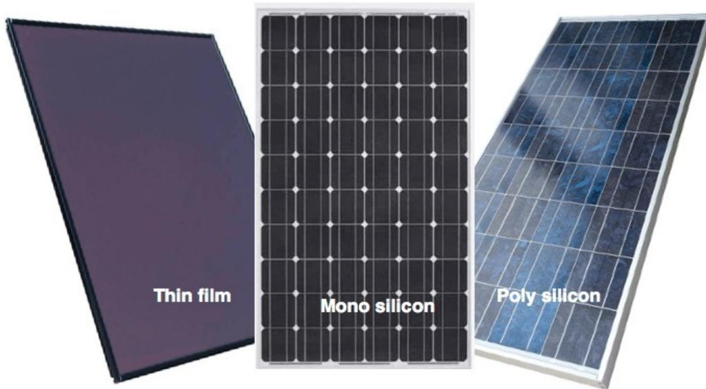
These are made using cells sliced from a single cylindrical crystal of silicon. This is the most efficient photovoltaic technology, typically converting around 15% of the sun's energy into electricity. The manufacturing process required to produce mono-crystalline silicon is complicated, resulting in slightly higher costs than other technologies.
