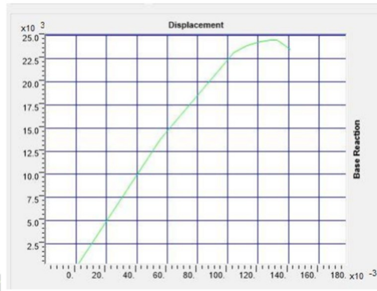
Fig 3: Pushover curve for model 1.
