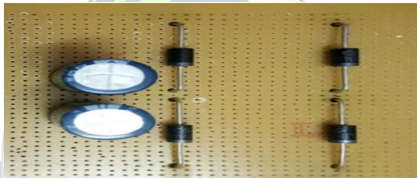
Fig.8: Secondary side diode bridge
