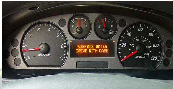
fig-1- LED Display on a dashboard of a car alerting the driver.
